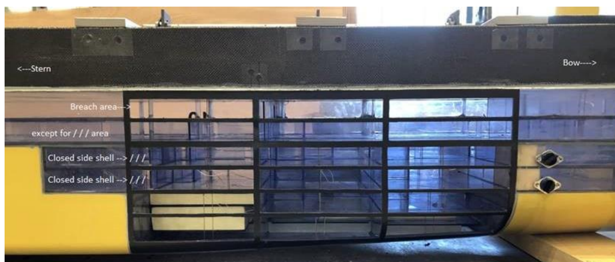
Figure 3 Breach openings in the SB side of the model (photo courtesy of MARIN).
