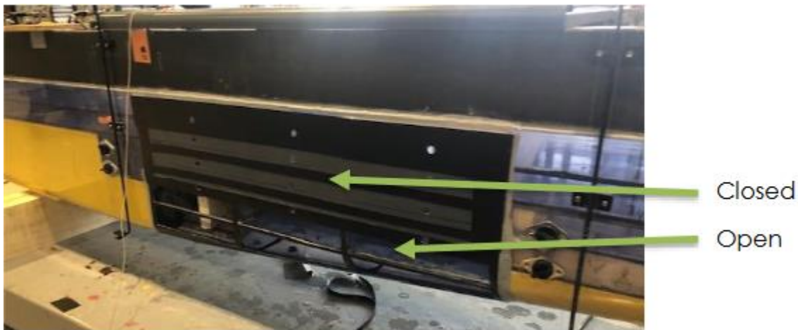
Figure 6 Breach in benchmark case 3 (photo courtesy of MARIN).
