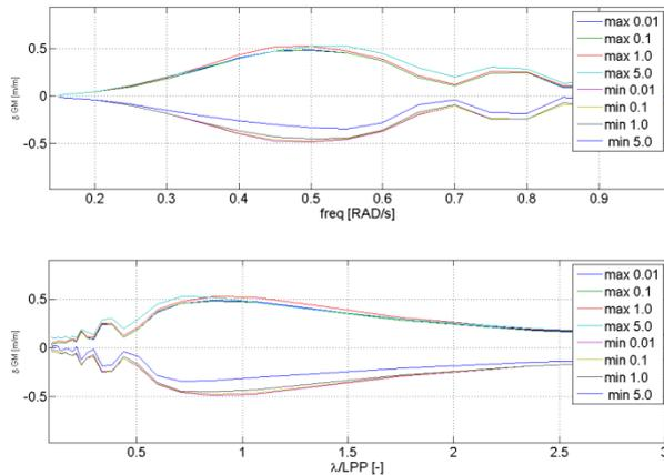
Fig. 6: Typical transfer function for the  $\delta GM$  as function of frequency (top) and as function of wave length over ship length  $\lambda/L_{PP}$  (bottom) for wave amplitudes between 0.01 and 5m.
