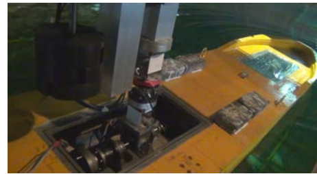
Fig.2 The ship model in partially restrained experiment
