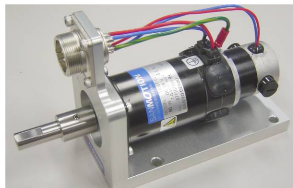
Fig. 3 – Propulsion motor (60W DC motor)
