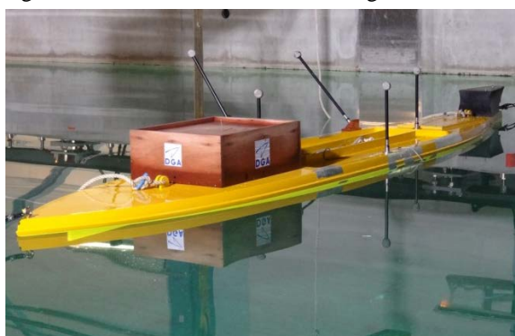
Fig. 12: Model during tests in the tank.
