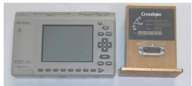
Fig. 7 –Data logger and 6DOF inertial sensor
