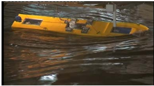
Fig.2 The ship model in free running experiment
