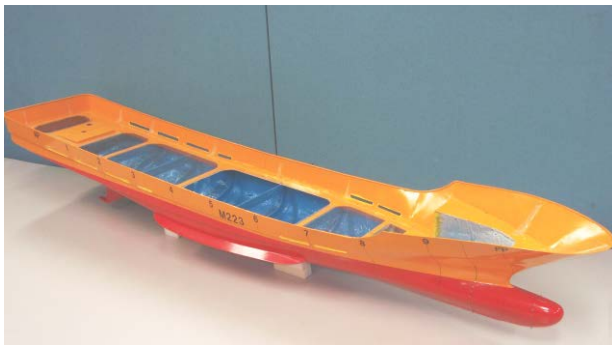
Fig. 1 – Ship model for free-running tests
