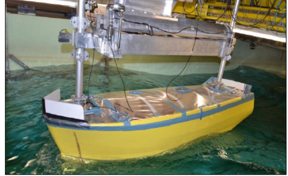
Fig. 8 - Surf-riding test while navigating on a wave crest
