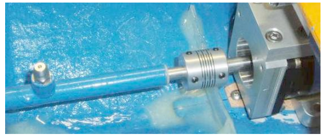
Fig. 4 – Connection of motor and propeller shafts
