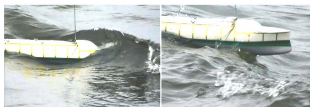
Fig. 4. Trawler hulls balanced by the lack of running trim in calm water, and this dynamic stabilization is not affected on a large stormy waves, where the motion of the wave energy goes mainly in heave, with no direct impact on the propulsive quality and stability on the storm course
