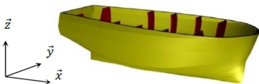
Fig. 1 - Hull shape of the model
