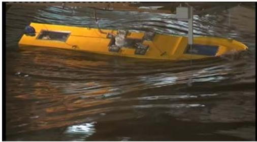
Fig.2 The ship model in free running experiment
