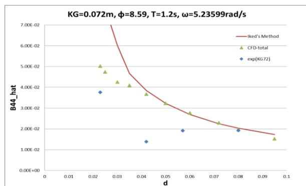
Fig. 7 – Dimensionless roll damping coefficient (KG=0.072)
