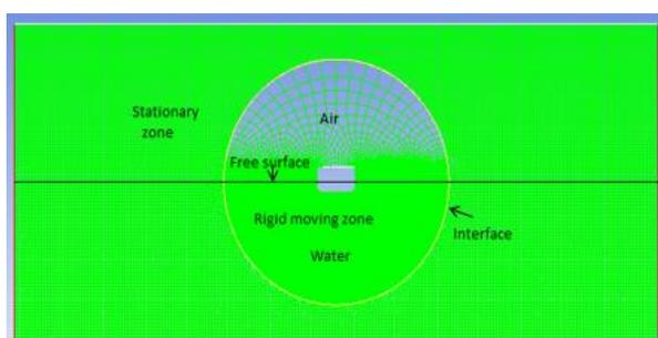
Fig. 3 – The geometry and computational mesh
