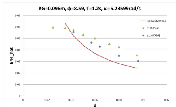
Fig. 8 – Dimensionless roll damping coefficient (KG=0.096)
