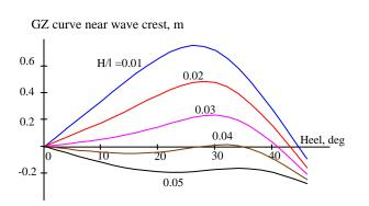
Figure 3 GZ curves in waves for different values of wave steepness, D=17 m with superstructure included
