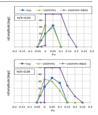
Figure 7: Comparisons of parametric roll between experiments and simulations, under the condition of  $\lambda/L_{pp}=1.0$ ,  $\chi=0^0$  and  $180^0$ .
