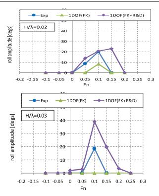
Figure 8: Comparisons of parametric roll between experiments and simulations, under the condition of  $\lambda/L_{pp}=1.0$ ,  $\chi=0^0$  and  $180^0$ .
