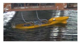
Figure 3: The passenger ship model in the free running experiment.
