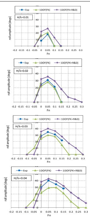
Figure 5: Comparisons of parametric roll between experiments and simulations, under the condition of  $\lambda/L_{pp}=1.0$ ,  $\chi=0^0$  and  $180^0$ .
