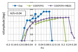
Figure 6: Comparisons of parametric roll between experiments and simulations, under the condition of  $\lambda/L_{pp}=1.0$ ,  $\chi=0^0$  and  $180^0$ .
