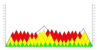
Figure 2: Example of color coding for flooding extent based on the floodable length curve.
