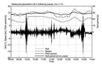
Figure 8: Sequence with the highest roll amplitudes during the studied 16-month period combined with 10 min average data for speed, pitch period and roll period. The periods have been plotted with different scales to better illustrate the excitation of large amplitudes when there is a perfect 2:1 relation between roll periods and pitch periods.
