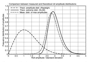
Figure 7: Distribution of roll amplitude extremes within 10 min records. N=56 corresponds to the average number of amplitudes to any direction within all records.
