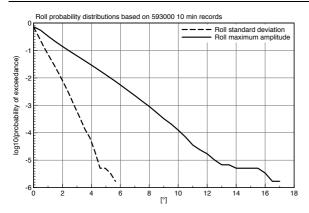
Figure 6: Long term distribution of roll standard deviation and maximum amplitudes within 10 min records from service data between June 2014 and September 2015.
