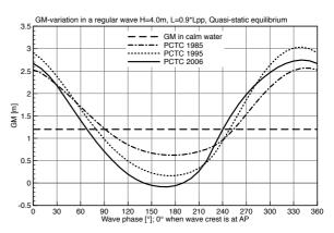
Figure 2: Comparison of three generation PCTC quasi static GM variation in regular waves. Wave height 4m, wave length 90% of Lpp.
