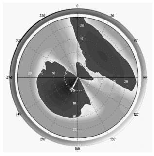
Figure 5: Example of heavy weather manoeuvring advise with regard to stability in waves in the on-board decision support system Seaware EnRoute Live.
