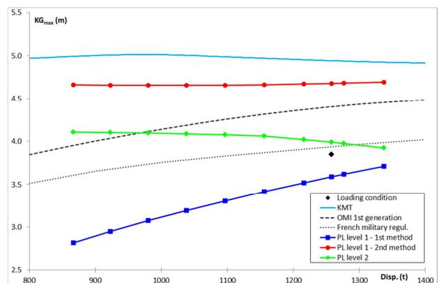
Figure 6:  $KG_{max}$  curves associated with the pure loss of stability criteria for the Offshore Patrol Vessel.
