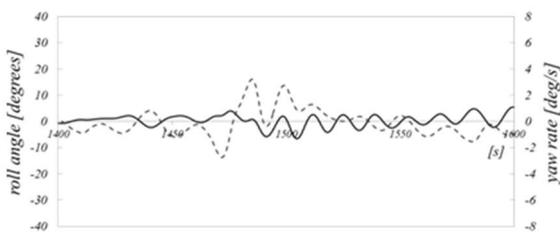
**Figure 4: Numerical simulation of the RoPax ship with the roll restoring variation and the coupling effect from sway and yaw to roll.**
