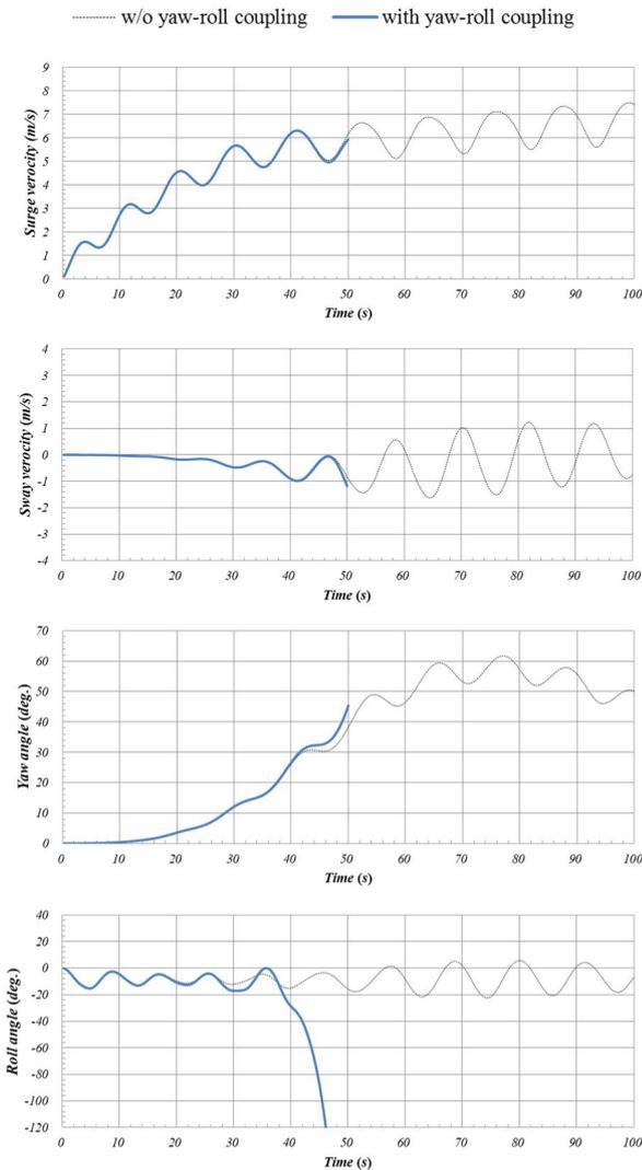
**Figure 8: Numerical simulation of the torpedo boat with and without yaw-roll coupling.** Here the wave steepness of 0.06, the wavelength to ship length ratio of 1.0, the Froude number of 0.26 and the heading angle of 50 degrees from the wave direction.
