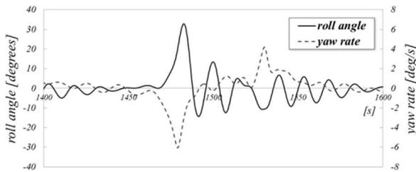
**Figure 3: Numerical simulation of the RoPax ship with the roll restoring variation and the coupling effect from sway and yaw to roll.**
