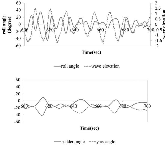
Figure 5: Numerical simulation of the ocean research vessel with the restoring variation.
