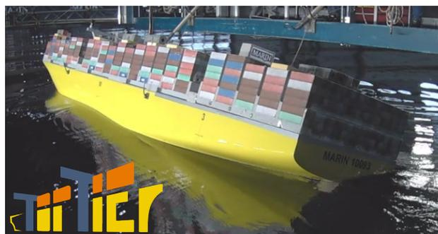
**Figure 2: Example of parametric roll in following seas for a 10,000 TEU container vessel (wave height 4 m, wave period 11.9 s, vessel speed 10.6 kn, max. roll angle 19.7 deg)**
