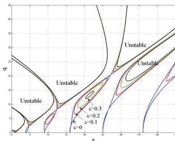
Fig.5 Stability chart for bi-frequency excitation for different damping ( $d=0.5$ )
