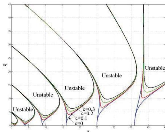
Fig.4 Stability chart for bi-frequency excitation for different damping ( $d=-0.5$ )
