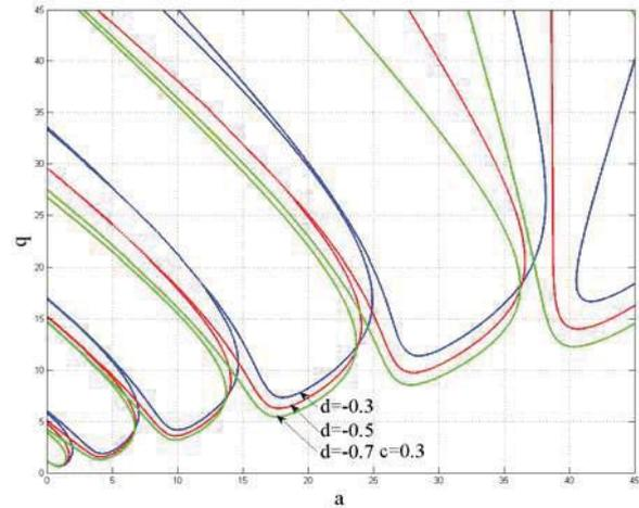
Fig.8 Stability chart for bi-frequency excitation for different d ( $c=0.3$ ) (Blue line-- $d=-0.3$ ; red line-- $d=-0.5$ ; green line-- $d=-0.7$ )
