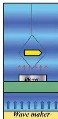
Figure 3 Overview of experimental setup (Umeda et al., 2014).
