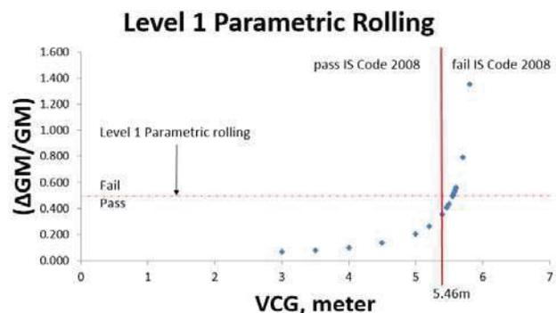
Figure 6 Result of Level 1 Parametric rolling
