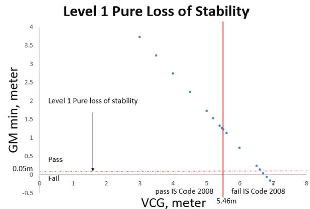
Figure 5 Result of Level 1 Pure loss of stability
