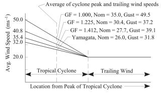
Figure 4 Simplified typhoon wind velocity, adapted from Yamagata (1959)
