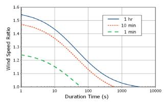
Figure 1 Wind speed ratio for 1 hour, 10 minute and 1 minute averaging periods
