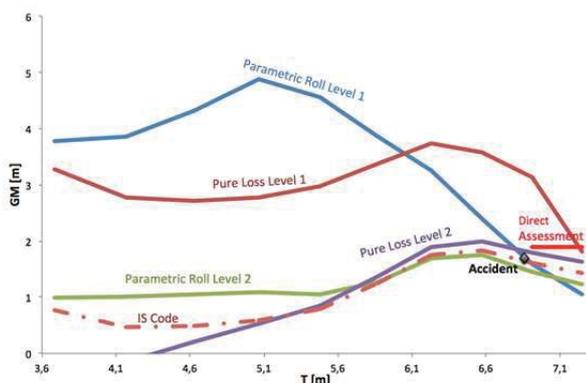
Figure 14: GM required curves for the RoPax 4
