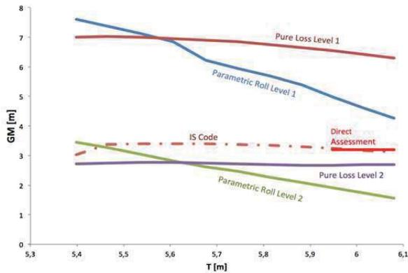
Figure 13: GM required curves for the RoPax 3
