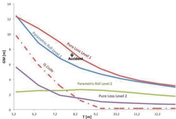
Figure 15: GM required curves for the Container 1
