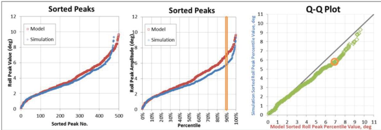
**Fig. 3** Sorted Peak Amplitudes for Two Data Sets [by number (left), by percentile (center), percentiles plotted against one another (right)]
