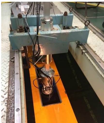
Fig.3 Towing rod and measurement system
