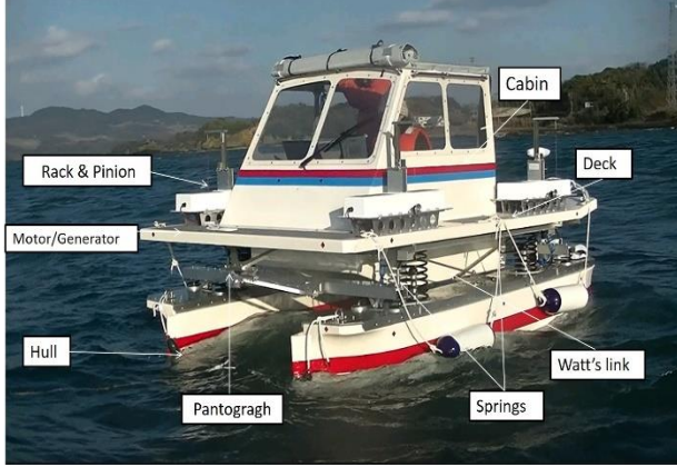
Figure 7 Structure and components of WHzer-7. The research was conducted during 2015-2016.
