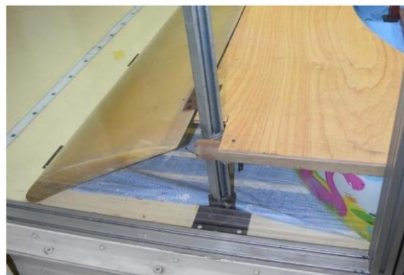
Figure 10 Side view of test section with spoiler and dummy test section floor
