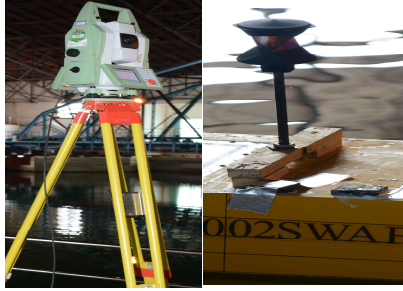
Fig. 2 The theodolite and the prism attached on the model ship
