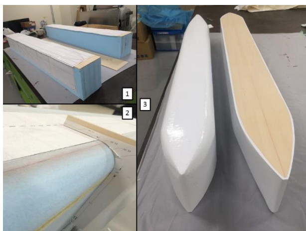
Figure 5 Steps of producing the displacement hulls. The research was conducted in 2013.
