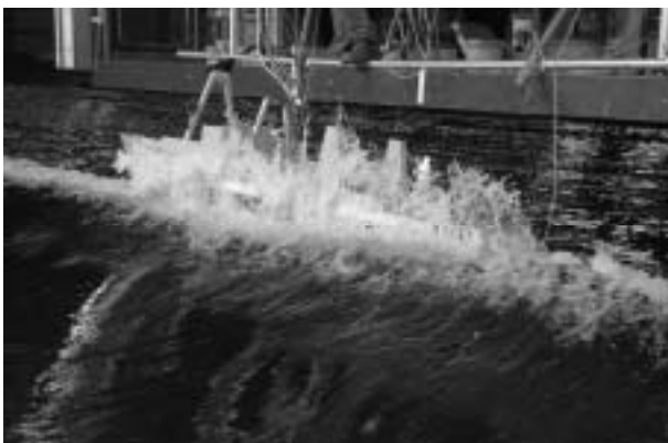
Figure 10 Gaul model in beam seas
