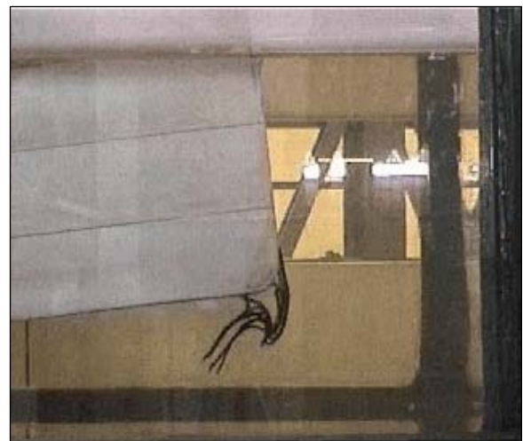
Figure 3. Strong vortex attracted to the hull bottom in the LARGE region (Oliveira, 2003).
