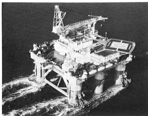
Photo. 1 A column-stabilized type semi-submersible platform
